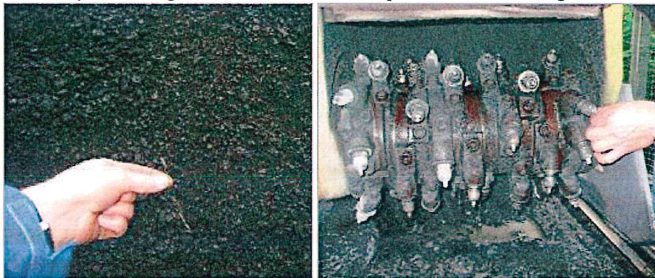
Figure 12: Residual fibres in the millings; few fibres remained on the milling drum
