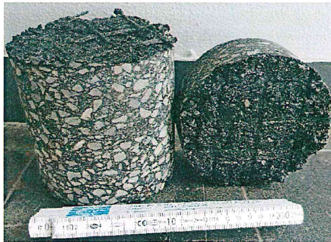
Figure 3: Drill core with reinforcement (after testing)
