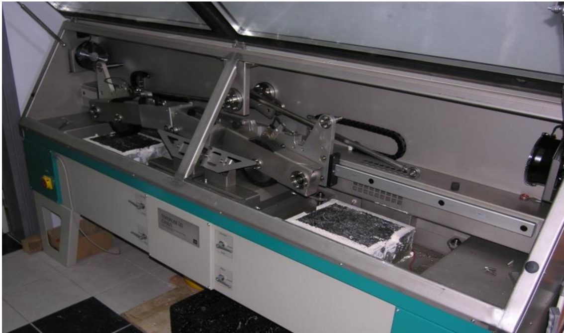
Rutting test of two identical specimens
