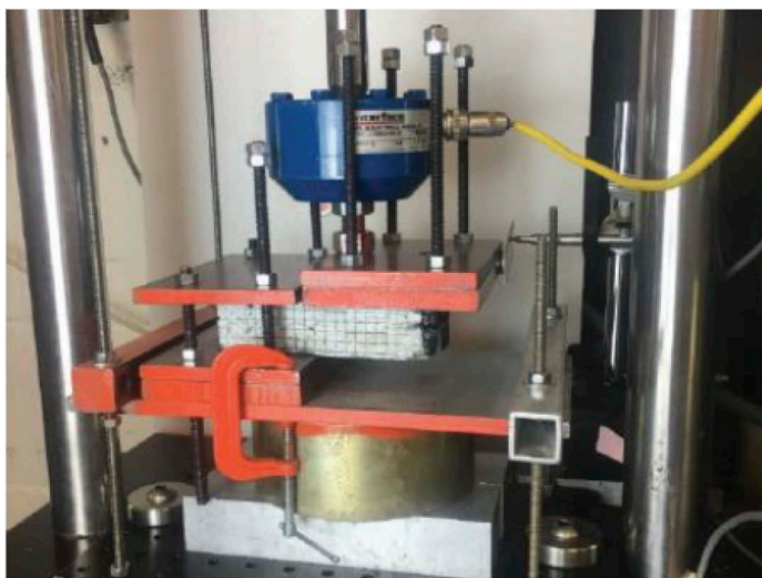
Figure 4. Test set up for shear fatigue test.
