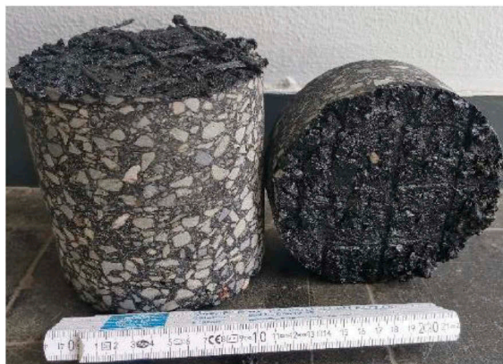
Figure 3. Drill core with reinforcement (after testing).
